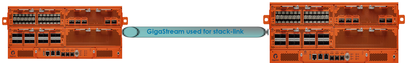
Figure 4 Daisy-Chain Configuration using GigaStream for Stack-link
